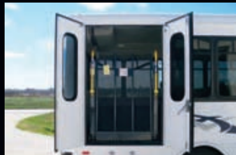
Optional double wheelchair door with top mounted gas shocks to hold door open in windy conditions
